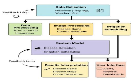
Figure 1.1: Work Flow of Crop Disease Detection and Smart Irrigation System
